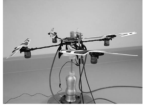
Fig. 3. Quadrotor aircraft experimental setup.
